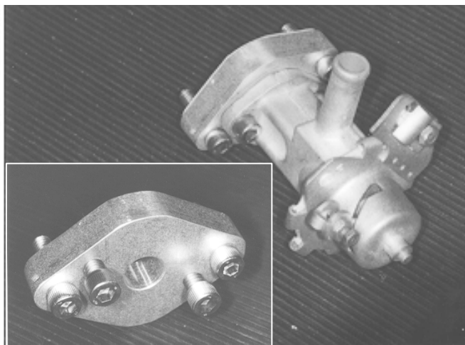
Top - MGB heater valve showing installation of D & D Fabrications new adapter kit. Kit shown in lower left.
